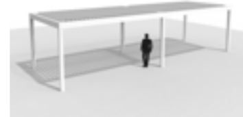
Two-part joined on the Span side
