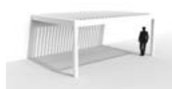
Façade mounting: the frame is placed with one or two sides against an underlying, supporting construction or structure. Vertical columns support the other part. The blades can be positioned parallel or perpendicular to the support structure.
